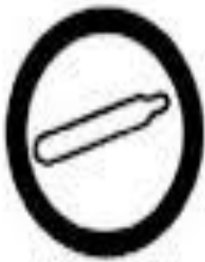
A - Compressed Gas
